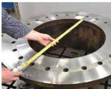
**5** Set machine onto flange using setup fingers. Lightly tighten leveling
